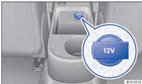
Fig. 160 Tomada 12 V no console central - variante 1.
