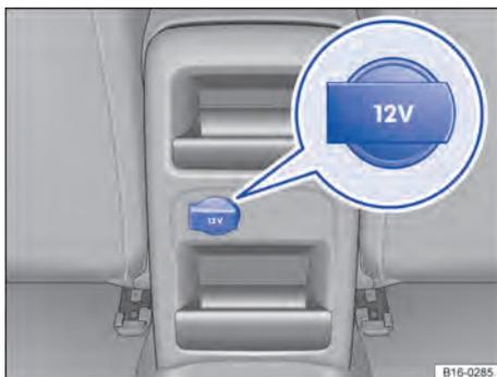
Fig. 161 Tomada 12 V no console central - variante 2.
