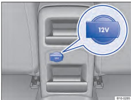
Fig. 131 Tomada 12 V no console central - variante 2.
