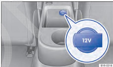
Fig. 130 Tomada 12 V no console central - variante 1.
