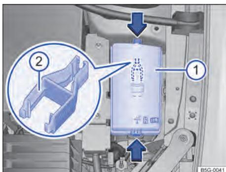
Fig. 171 No compartimento do motor: cobertura
